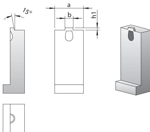
**EN** The companion vestige and/or dead-end recess can also be incorporated directly in the mould insert. The auxiliary insert should be made of a highly wear-resistant steel.
