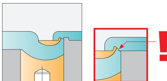
**EN** For optimum degating (especially of flat parts), we recommend the use of a companion vestige supplementing the vestige with cutting edge. This configuration will ensure that the part is separated from the runner flush with the parting line. Users will find this particularly advantageous in cases where materials are susceptible to stringing.
