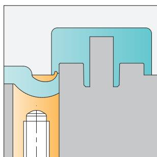
**flat part with companion vestige - installation in fixed half of the mold**
