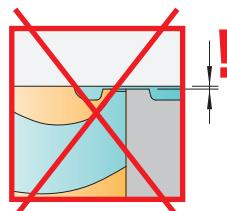
**EN** For optimum degating (especially of flat parts), we recommend the use of a companion vestige supplementing the vestige with cutting edge. This configuration will ensure that the part is separated from the runner flush with the parting line. Users will find this particularly advantageous in cases where materials are susceptible to stringing.
