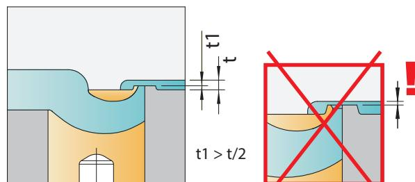
**EN** If the molded part is very thin, the calotte must be ground down. ( $t_1 > t_2$ )
