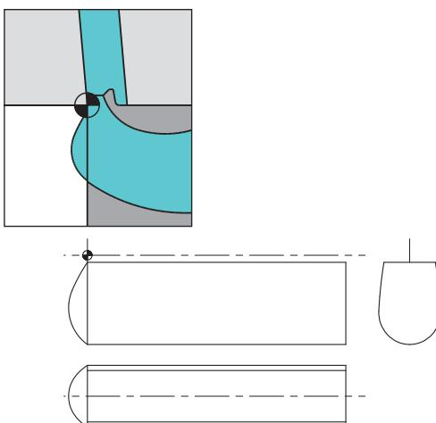
**EN** When machining the recess, take care to avoid undercutting the runner. For 3D data relating to standard insert sizes please refer to [www.i-mold.com](http://www.i-mold.com) (download section).
