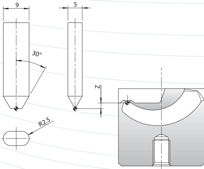
**EN Gate machining by spark erosion**
