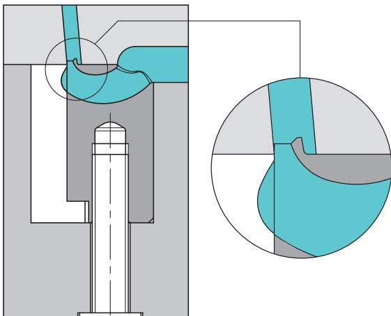
**EN** For the gating of housing parts we recommend incorporating a dead-end recess in an auxiliary insert or directly in the mould insert. This feature optimizes the shear velocity in the gate area, gives a superior frontal flow, reduces the pressure loss and helps prevent jetting.
